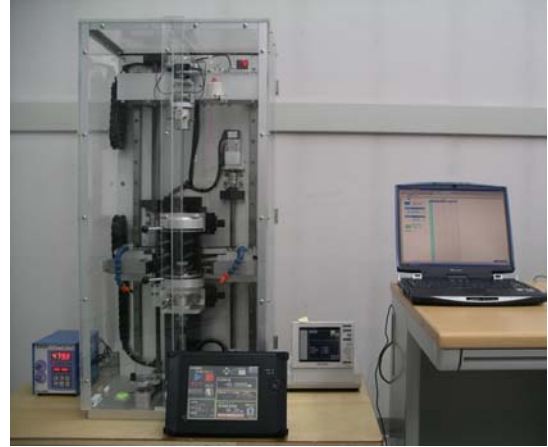
Fig. 2 Diameter measurement system for air lines
